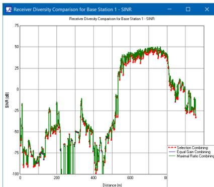
Figure 3: SINR comparison of receiver diversity methods for base station 1.
