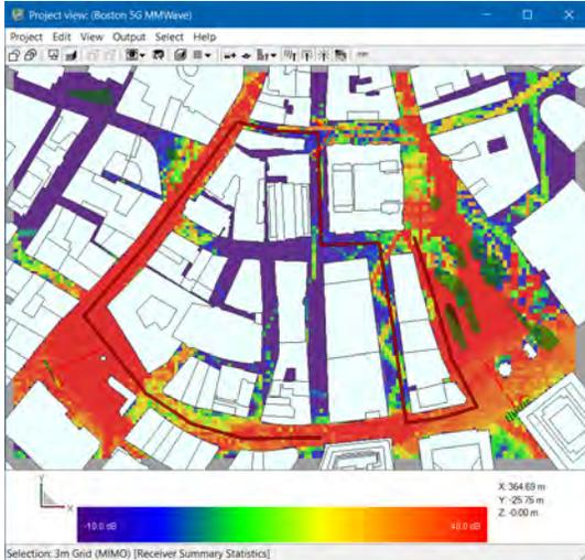
Figure 9: SINR coverage for custom beamforming and selection combining.
