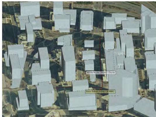
*Figure 1: Rosslyn 3D building and terrain data are set up for SISO and MIMO analysis within Wireless InSite.*
