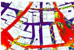
**Example 5: Throughput of a 5G New Radio FD-MIMO System in an Urban Area Using Custom Beamforming**
