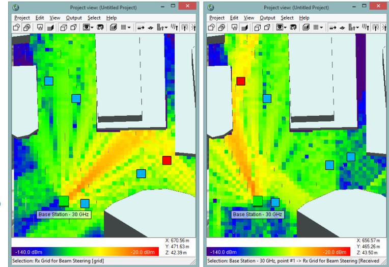
Wireless InSite showing how multipath could influence beamforming to > one device
