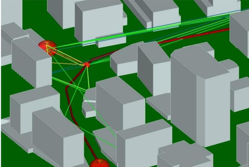
Small-scale fading from multipath causes rapid fluctuations along route
