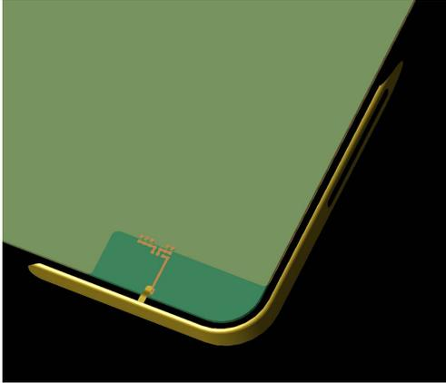
Figure 4: Layout of matching network.
