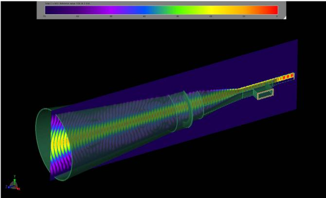
Figure 8: At 340 GHz, the time domain electric fields are more tightly bound to the tapered dielectric strip in the center of the horn.
