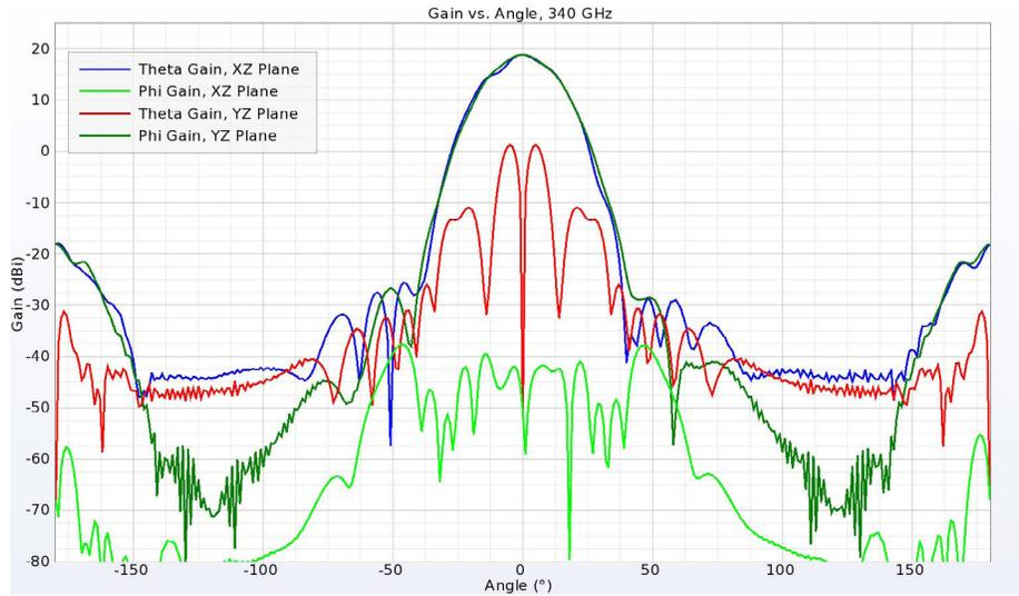
Figure 13: At 340 GHz, the gain in the principal planes is symmetrical with low side lobes. The cross-polarized fields are higher in one plane but are still down more than 15 dB.
