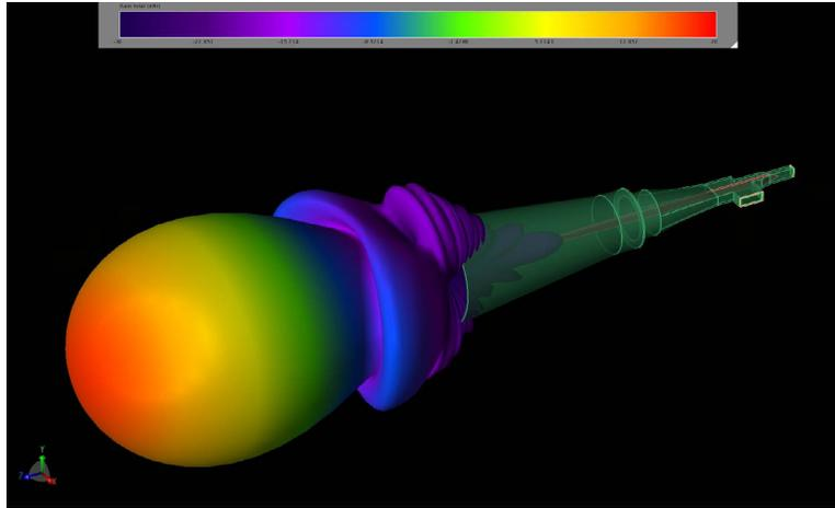
Figure 10: The gain pattern of the horn at 94 GHz has a symmetrical beam with peak gain at 18 dBi and low side lobes.
