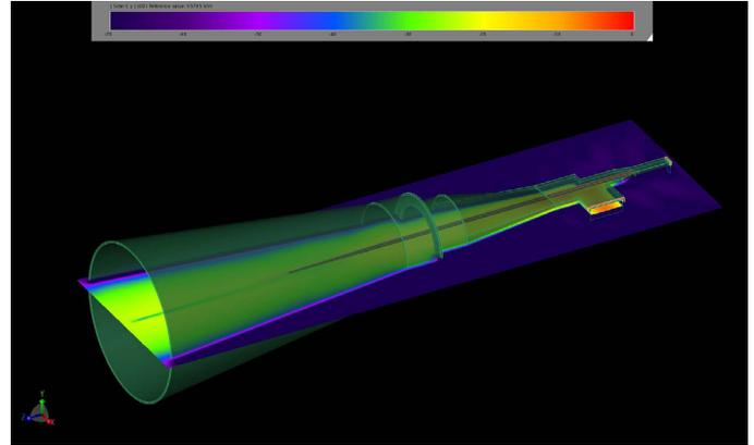
Figure 7: Steady-state electric fields at 94 GHz show field distributions throughout the cross section of the horn.
