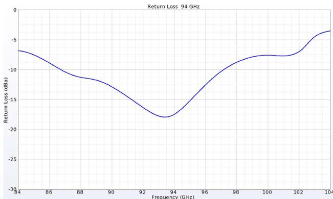
Figure 4: The return loss for the 94 GHz port shows a good match with values below -15 dB.
