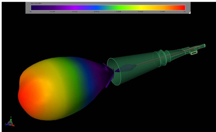
Figure 11: At 340 GHz the gain pattern has a nearly-symmetrical beam with a slightly higher peak gain of nearly 19 dBi. The sidelobes are down nearly 40 dB from the peak.
