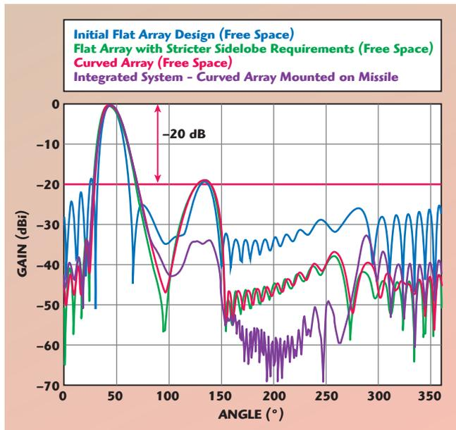
▲ Fig. 3 Optimized simulated antenna gain vs. angle.
