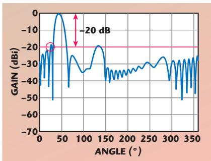
▲ Fig. 2 Simulated antenna gain vs. angle.
