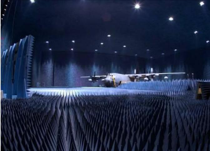
Figure (2) MC-130 under test at the BAF, Edwards AFB
