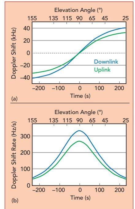
▲ **Fig. 2** Doppler shift (a) and Doppler drift rate (b) for a satellite in LEO orbit.
