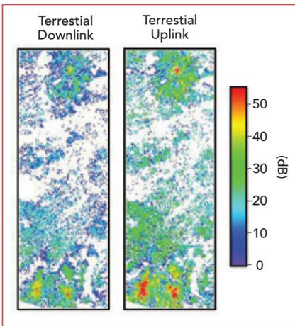
**▲ Fig. 4** NB-IoT SNR for a terrestrial downlink and uplink.
