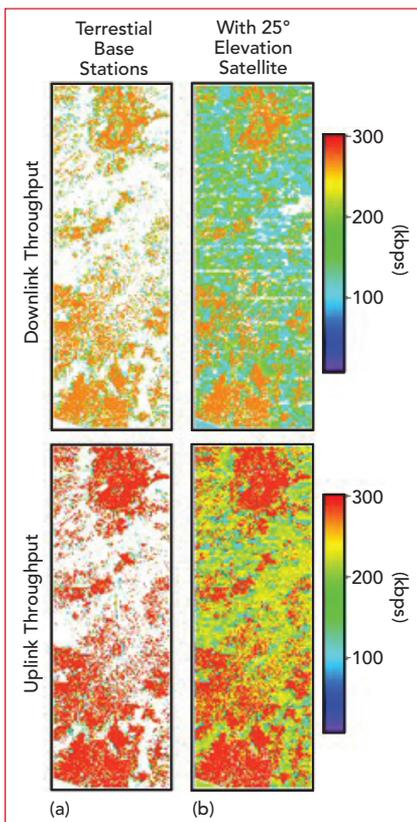
▲ Fig. 7 NB-IoT downlink and uplink throughput, comparing the terrestrial base stations (a) vs. satellite overlay (b), with the satellite at 25° elevation.
