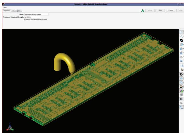
▲ Fig. 3 Definition of dielectric breakdown sensor.
