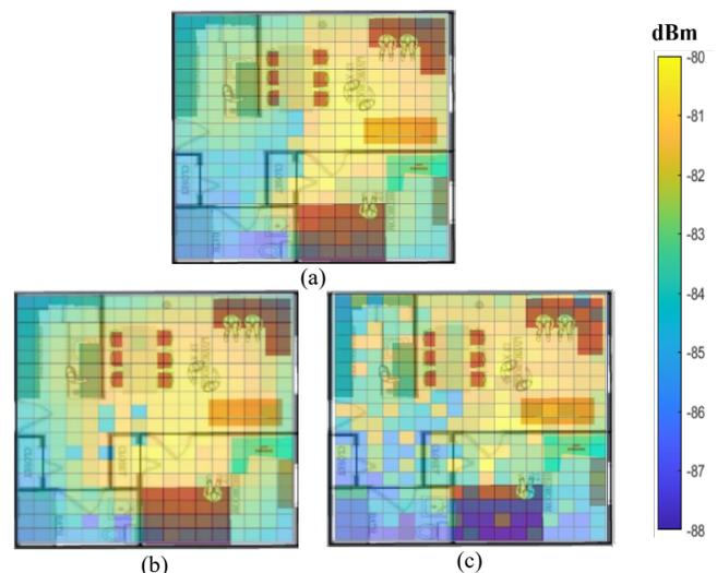
Fig. 4. Average signal power corresponding to the position of transmitter, obtained by: (a) Wireless InSite; (b) NN; (c) MR. The transmitter should be placed in the bright yellow regions for best overall coverage.
