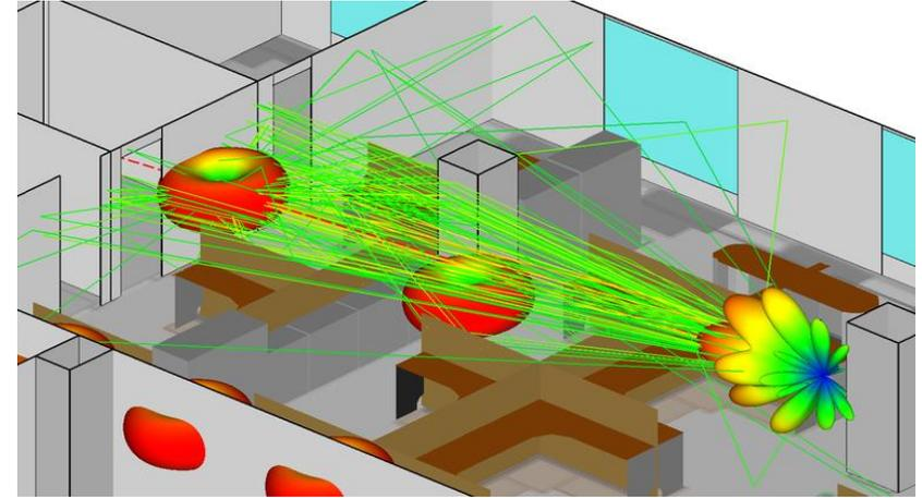
Predicting channel characteristics for macrocells, small cells, and indoor Wi-Fi
