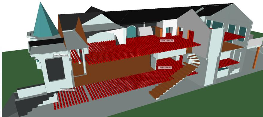
Figure 2: Receiver grid used for studying throughput coverage.
