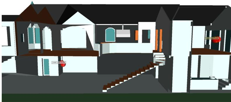
Figure 1: Locations of the transmitting routers (red far-field patterns) within the house geometry.
